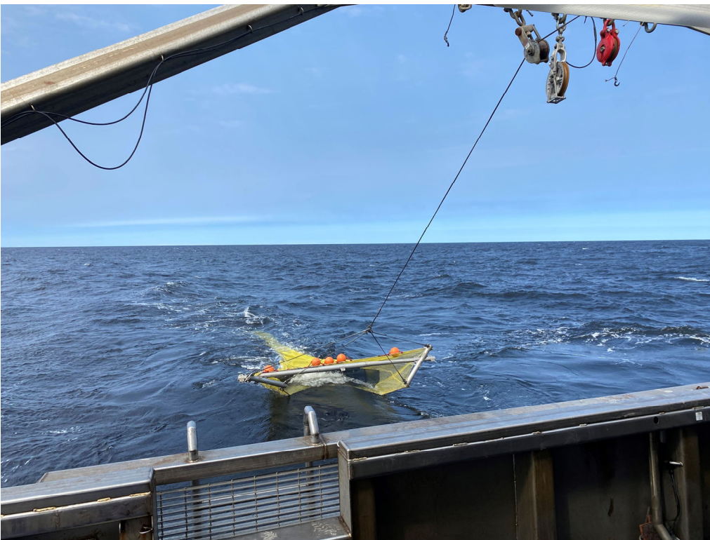
Figure 22. Benthic beam trawl being deployed over the stern.
