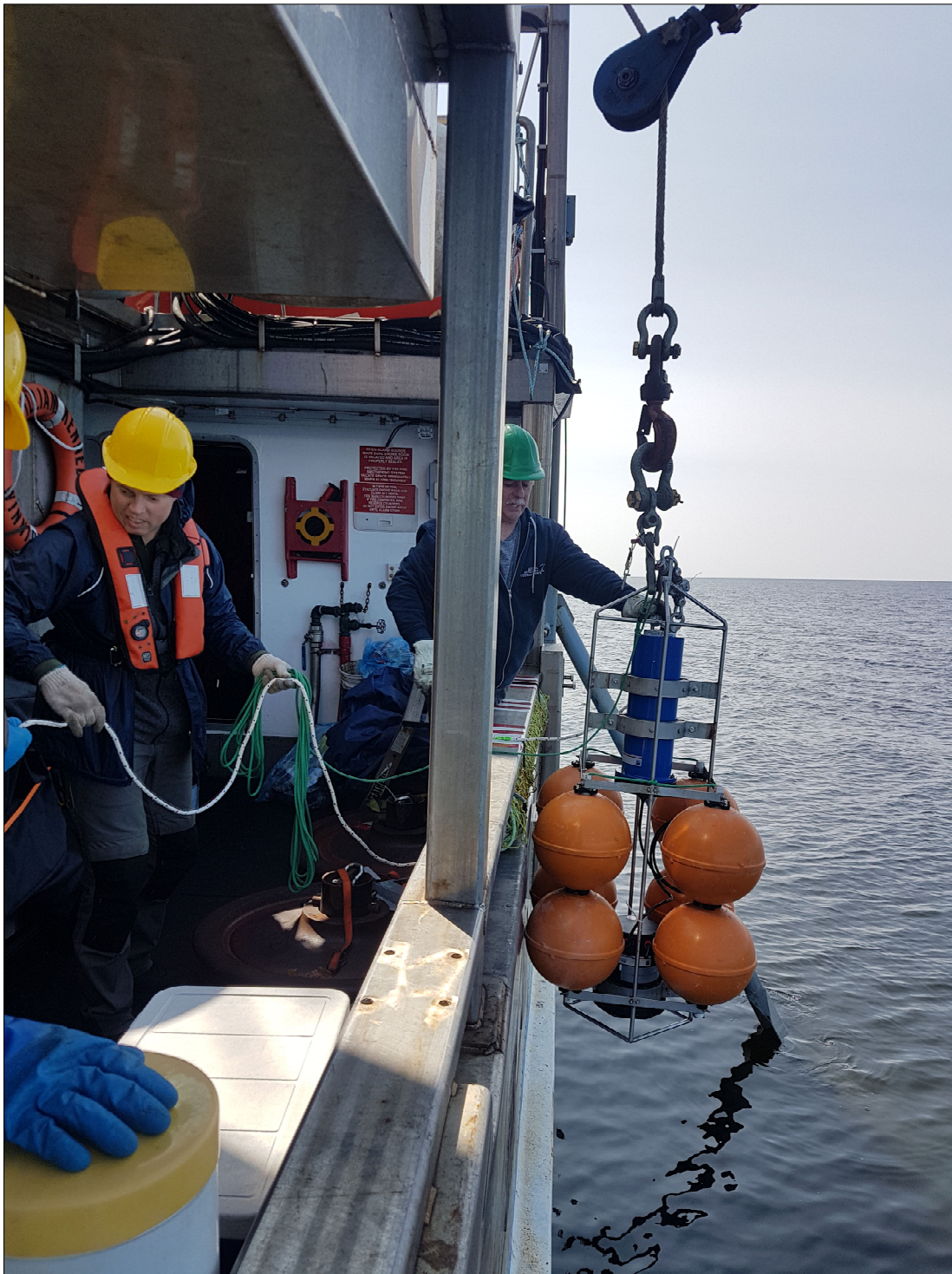
Figure 11. Deployment of the Nortek Signature 500 ADCP and upward looking sonar as part of the JB-M5b mooring on 8 August 2021.
